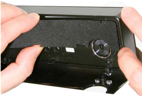
Installation of the self-adhesive mylar
